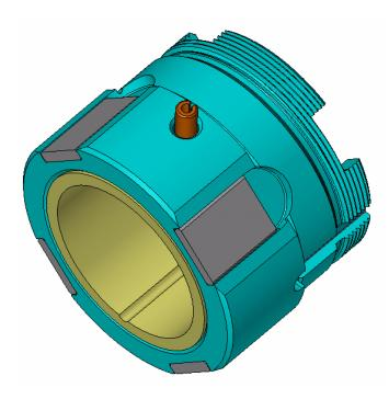
This is a re-design of our standard 5080-131 Clutch Body. The new **Roll Away Clutch Body** now accepts 4 hardened wear plates. These wear plates can be flipped end over end, and spun around on each side, exposing 4 different wear zones per plate to the roller load.
