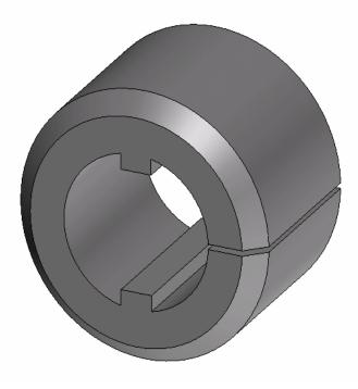
The redesigned **Clutch Body** is now slotted through the side. This allows the **Gripping Sleeve** segments to collapse the **Clutch Body** onto the shaft, greatly improving the torque capacity of the threading clutch unit.
