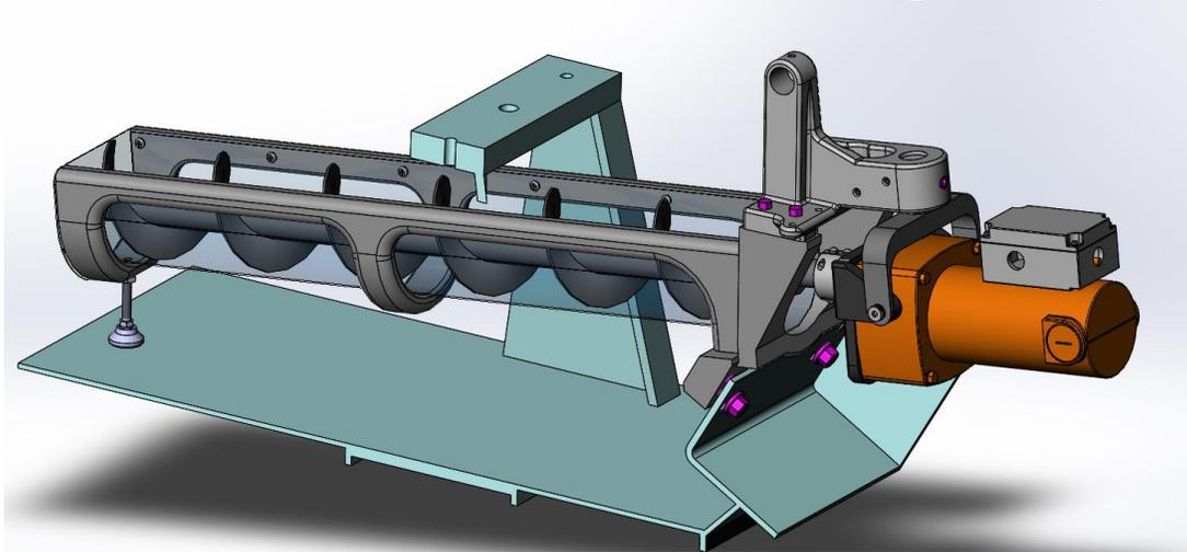
The *5080-329-78-SA Motorized In-Line Chip Conveyor* is a direct-drive, in-line motorized replacement for all previous generations of auger-style chip conveyors, including ratchet driven, as well as previous right-angle motorized chip augers. It is available as a replacement part for existing machines, or a factory installed option on all new Model-B and HP machines. The low-profile design clears all existing components, enclosures, and access points.
