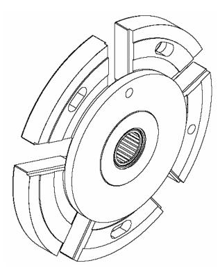
The redesigned **Geneva Motion Star Wheel** now uses a precision needle bearing instead of the traditional bronze bushing. Wear of the bronze bushing over time can cause inconsistent indexing of the revolving head, and is a leading cause of revolving head crashes. This machine failure can be particularly difficult & costly to repair. Severe crashes usually crack a rib on the revolving head, and may require the complete disassembly of major sections of the machine, and costly repair parts.
